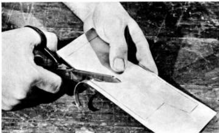
Figure 1 SOFT ALUMINUM SHEET MAY BE CUT WITH HEAVY KITCHEN SHEARS
